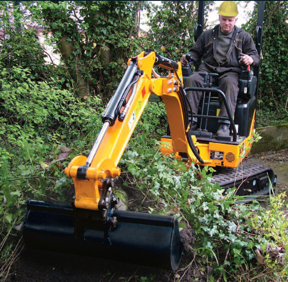
Side-mounted joysticks allow a clear view of the working area from the operator's seat.
