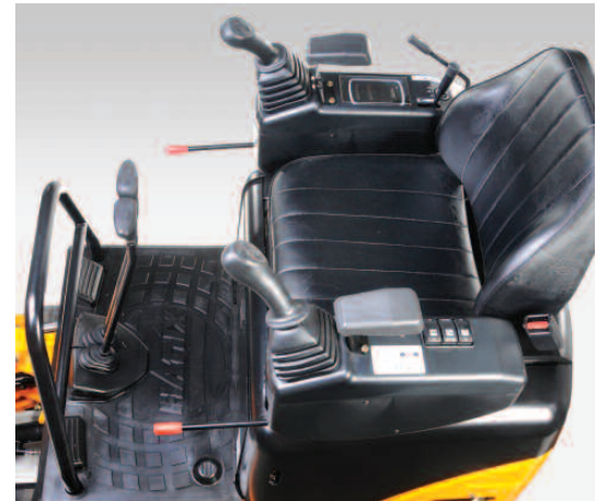
Well-appointed operator's station with all controls easily to hand.
