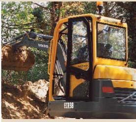
Open door is protected within the swing radius of the chassis.
